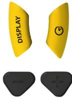
**Press and hold the 'DISPLAY' and 'CLOCK' buttons for 3 seconds.**
